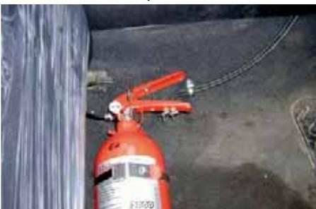
Remember that FIA-homologated extinguishers systems must be "secured by a minimum of 2 screw locked metallic straps and the securing system must be able to withstand a deceleration of 25g" [FIA Appendix J 253-7.2.2]. With any installation, check that the extinguisher will be retained. Extinguishers are 5kg or more and will do a lot of damage if they come free in an impact.
