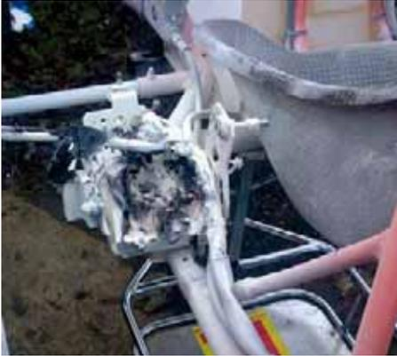
igniting is unknown; strictly speaking it is not a fire but an exothermic reaction. It generally occurs when the battery is overheated by excessively high discharge or recharge rates, or by an internal shorting as a result of fault or mechanical damage.
