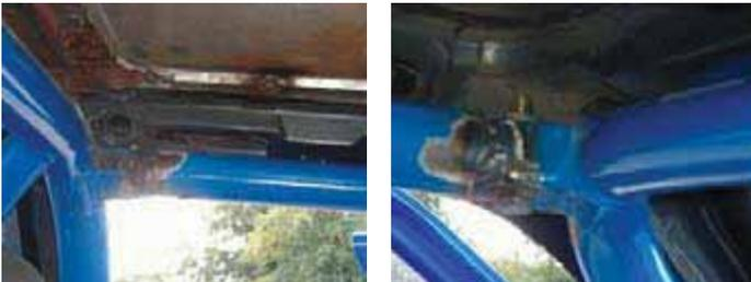
However, (K)1.3.7 states: *“Demountable joints must not be used as part of the main, front or lateral rollbar because they act as hinges in the principle structure and allow deformation. Their use is solely for attaching members to the rollbars and attaching a lateral rollbar to a main rollbar (see drawing K2) in this last case, hinged joints in drawings K21 to K30 must not be used”.*
